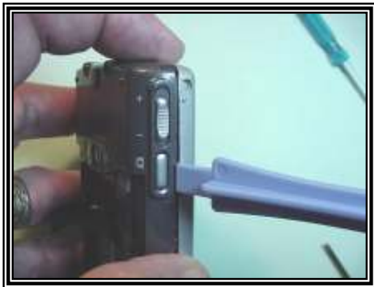
Insert Case opening tool between front bezel and rear cover to release plastic snap detail that holds them together. (Continued on Page 2)
