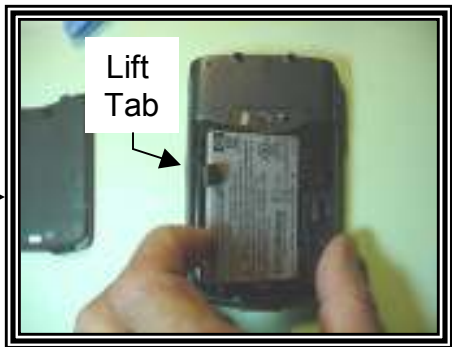
Using pull tab at left edge, lift and remove battery.
