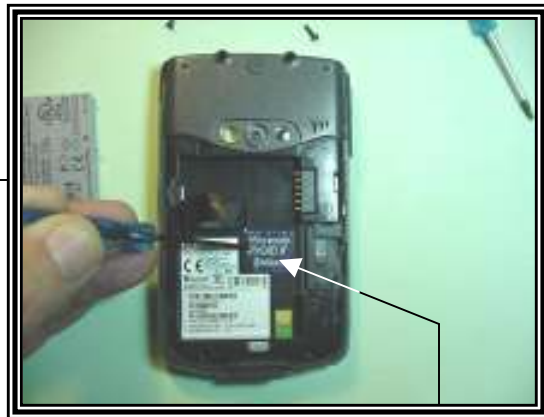
Using Philips Screwdriver, remove single silver colored screw located under "Warranty Void if Broken" label.
